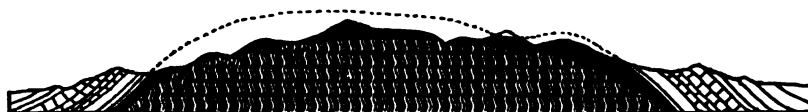
FIG. 17.—Section of interformational laccolith, Little Rocky Mts., Montana. (W. H. Weed and L. V. Pirsson, Jour. Geol., Vol. 4, 1896, p. 412.) Solid black , laccolith; roof , Paleozoic sediments; floor , pre-Cambrian schists. Length of section about 10 miles (16 km.).
